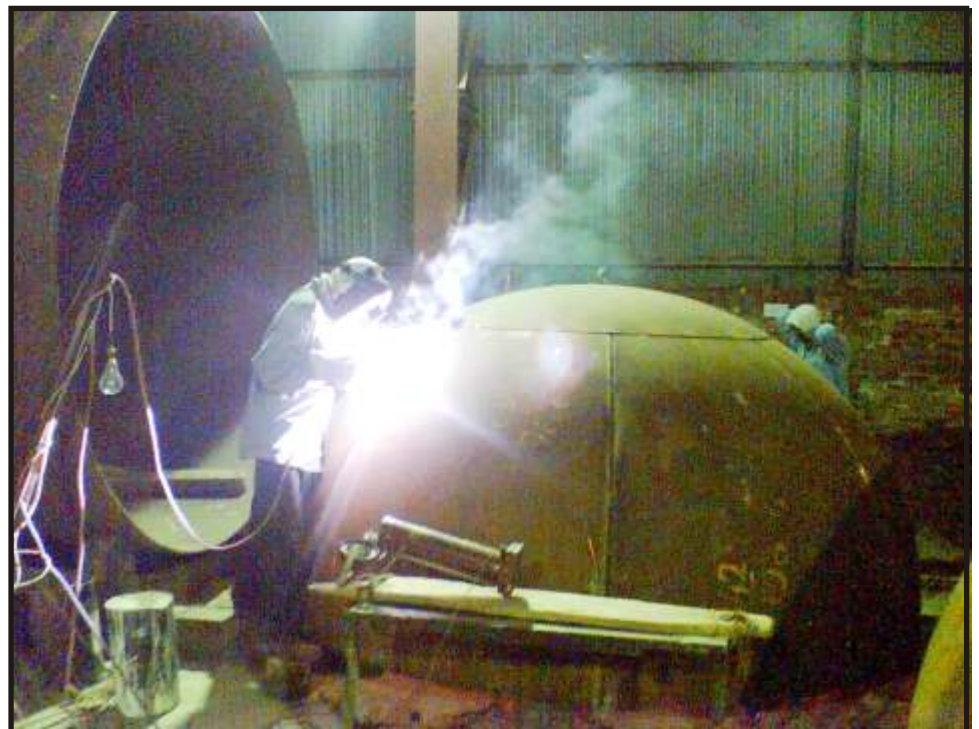
HEMI SPHERICAL HEAD WELDING
